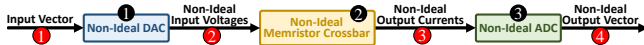
Figure 4: An overview of the VMM Model Generator's second approach: using analytical models.
